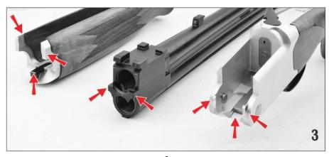
**3**. Attach barrels to the action by pushing the top lever to the right and engaging the dual hinge pin bearing notches on each side of the barrel. Hold the barrels with the muzzle at a downward angle with respect to the receiver. Once the bearings are properly seated, lift up on the barrels and close the action
